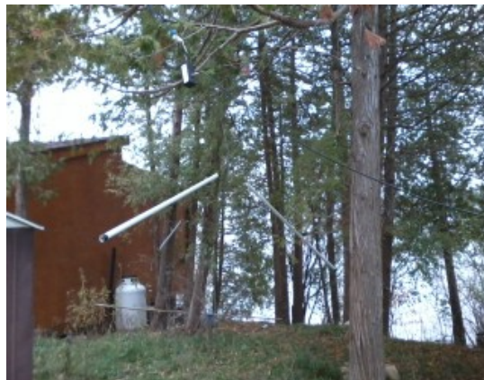
Photo 1: One of the author's loaded inverted vee dipoles
