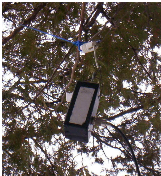
Photo 4: A completed Magnetic Longwire Balun (MLB)
