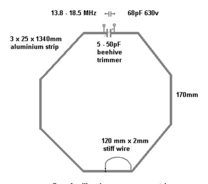
Coax feedline: inner = gamma match, braid = centre of bottom side
