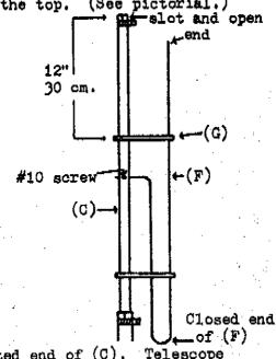
the two clamped sections will lower resonance. Shortening will raise resonance. Adjust one section at a time very carefully, repeating several times. Ordinarily adjustment will not
