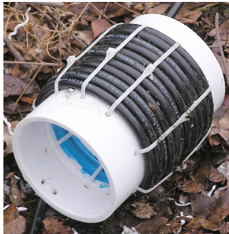
Picture above courtesy of KC2NXV (now N4NYY) shows using 2 pvc couplers joined and glued using about 2 inches of 4 inch PVC pipe, so the couplers would adhere and be stronger.
