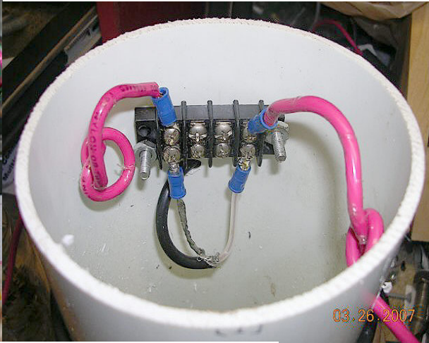
Photos courtesy Bill, KI4PCB, using 4 " PVC FORM Notice the screw terminal block used for connections
