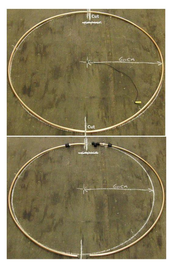
The 15 mm diameter soft copper tubing (from a hardware store) is 4 meters long, actually there are two easy to bend pieces of 2 meters.
