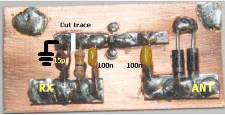
The INA 02186 has a high gain and a good connection to ground is essential. Some home brewers had to deal with an oscillating amplifier. To prevent instability ensure that both lips have direct contact with each other via one track. Do not separated by a machined groove, but solder on the same "island" or track.
