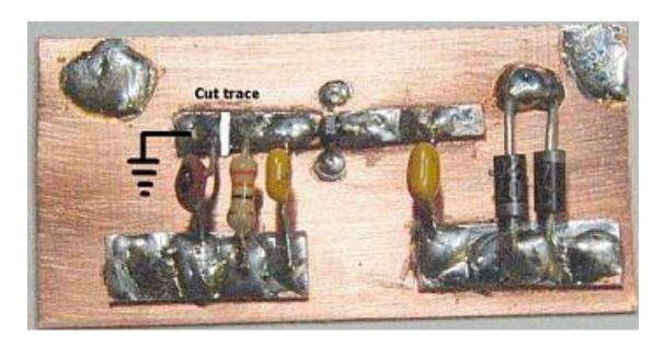
Slide the amplifier in the 22 mm-copper tube. Solder the mass of the PCB with a suitable soldering iron on the inside of the tube. Also use that point for one side of the flexible wire. Solder the other side of the wire to the input of the amplifier.
