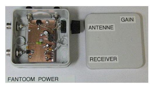
In previous schematic 330 ohm resistor was 240 ohm. Sometimes the IC was oscillating with short coaxial cable, therefore the resistance was increased and IC's supply voltage was reduced to 5.5 volts.
