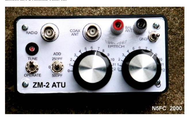
The Emtech ZM-2 Antenna Tuner is a nifty little portable transmatch for QRP (low power). It utilizes the well-known Z-match circuit, which is especially useful for balanced antennas (like dipoles and loops). Since it's a very inexpensive kit (around \$50), and because there's an constant clatter about it on the QRP-L mail list, and because I travel a lot and need the miniature equipment, I figured it would be worth investigating.
