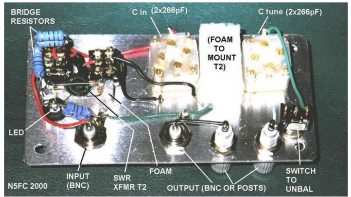
One thing to notice is that I've placed small foam blocks (from scrap packing material) to mount the transformers so that they'll stay in place. Here, we used the XYL's hot-glue gun to stick these down (and we'll do the same to mount the toroids). Here's another detail of the input circuit, showing the 3-D components and the SWR transformer T2 mounted on a little piece of foam:
