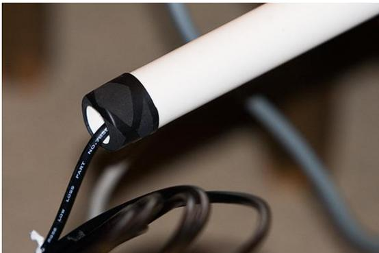
Heatshrink the bottom end to provide a buffer for the exiting coax and neaten the base.
