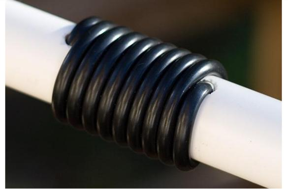
Image 11 – choke, note 9turns & mark visible at hole
