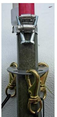
At left – the two small bolts clamped to the top of the mast fit around the clamp on the wooden dowel so that it cannot rotate in the wind. The antenna can be rotated by twisting the entire mast, the steel guy collar easily slips on the mast. I apply vinyl tape to each joint of the mast sections during assembly to keep them locked together.
