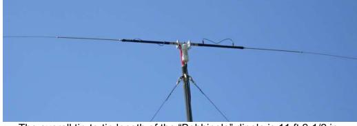
The overall tip-to-tip length of the "Bobbipole" dipole is 11 ft 2-1/2 in.
