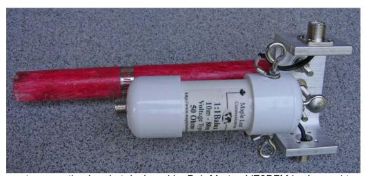
Here, the center mounting bracket designed by Bob Morton VE3BFM is clamped to a one foot piece of 1-3/16" painted hardwood dowel which fits into the end of the top mast section – a pipe clamp keeps it from sliding all the way in. Construction of the center bracket-balun assembly is very sturdy and can accept masts up to 1-1/2 inch, all connectors are SO-239.
