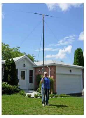
Jack VE3RDQ stands beside the Bobbipole mounted on a 16 foot guyed mast (since the 4 foot mast sections plug into each other 3-1/2", the actual height of the dipole was 15ft 8in). A 75 foot length of RG8X coax leads into the house for some testing.
