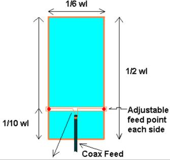
Center conductor to one side, shield to other side 1/10 wavelength up from narrow wire section.
