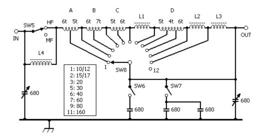
Lack of space in the box required the use of space-saving coils wound on plain 0.1 inch matrix board. Coils A and B were each wound on the matrix board in the form of a solenoid. Coils C and D were also wound on matrix board, but were wound 'flat'. Coils L1; L2; L3 and L4 were wound on T50-2 and T80-2 ring cores (see below).
