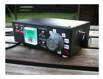
The ATU is built into a matt black box of ABS plastic having external measurements of 198 x 112 x 64 mm (Maplin part number BZ75S).
