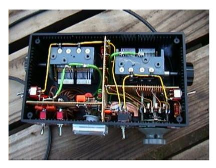
The above picture shows how I mounted the variable capacitors in an opposing configuration. Ideally, the panel knobs would be forward-facing, but the size of the box would not permit such luxury! Nevertheless, I have become used to adjusting the matching unit, and no longer find it tedious to adjust the side-mounted controls for the best match (i.e. minimum meter deflection while in the TUNE position).
