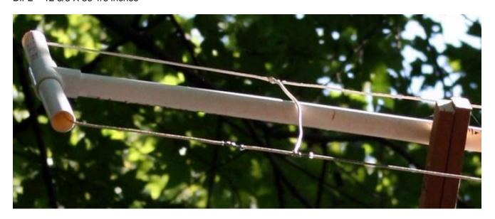
Shown above is the typical matching method using shorted feed points on the director #2 as an example. The reflector, and director #1 were done the same way. The driven element is fed with coax at it's respective matching point.
