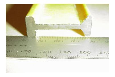
I wanted this antenna to be portable, so the elements needed to be removeable. I did this by machining bushes for the directors from 19mm aluminium bar and glued these to the boom using epoxy resin. The following photos (hopefully) show enough detail of these bushes. The clamping screws happened to be some from the junk box, but anything with a diameter of about 3mm should do the job.
