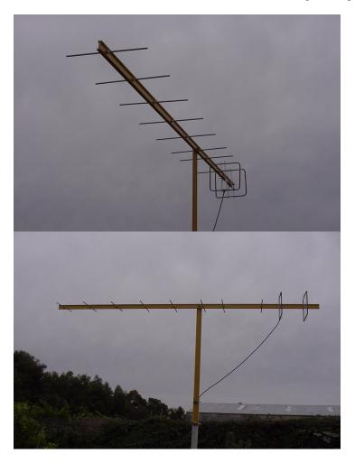
Materials used were 6mm (1/4 inch) aluminium rod for the directors, 6mm copper tube for the quad elements, 6mm polycarbonate (LEXAN) sheet for the quad spreaders, pultruded fibreglass boom, machined aluminium bar for director mountings.
