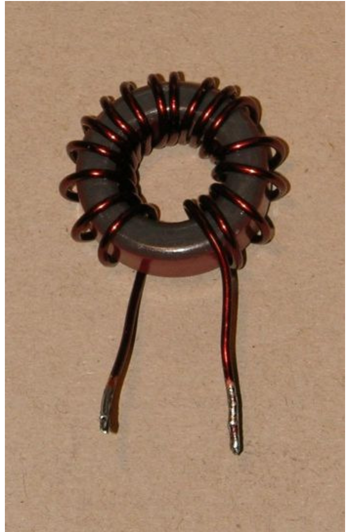
16 1/2 turns wide spaced give an inductivity of 2,5 uH
