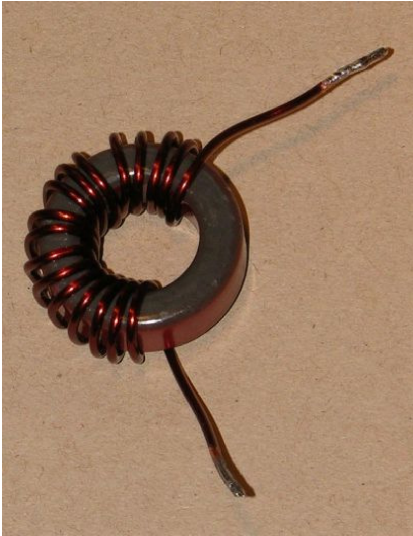
16 1/2 turns close spaced give an inductivity of 2,8 uH
