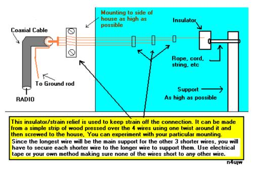
Note: In the instruction box above, the last sentence refers to the long portion of the wires, not at the connection point to the coax feed line to the receiver. All wires are connected together at the connector center conductor wire!
