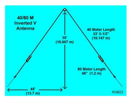
The forms for the loading coils are made of 1-1/2" (50 mm outside diameter) Schedule 40 PVC pipe. You will also need some 18 gauge magnet wire (available on the internet in one pound spools) and some number six stainless steel hardware. There are 78 turns of magnet wire on each loading coil.
