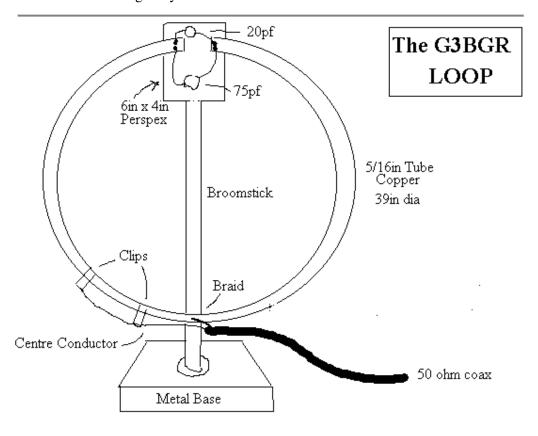
This ia a home built Magnetic loop antenna which was used by G3BGR, indoors on 7,10 and 14Mhz. The basic idea was in Radcom 1986
