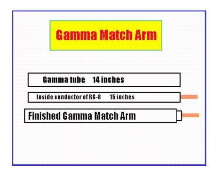
The gamma match is made from 3/8 inch tubing.
