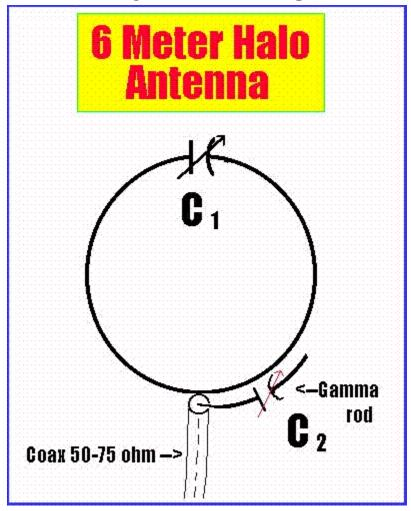
The 6 meter Halo is a good antenna that can be used for the car as well as the house. This antenna maintains good omni-directional horizontal polarization.
