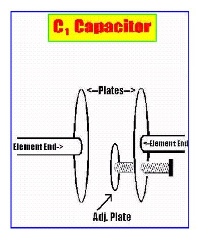
The 2 large discs can be about 4-5 inches round and the small disc about 1.5 inches. Mount the 2 larger discs at the ends of the halo by screwing end caps to the center of them and then the end caps will go over the ends of the halo.
