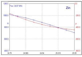
The SWR and Impedance graphs show that the G7FEK has a very high input impedance >1000 ohms (SWR 20.4: @ 24.77 MHz) on the 12 m band, but was still tuned using a Welz Antenna Matcher & MFJ 945E "T" match tuners. The antenna produces a clover leaf pattern of Horizontal lobes. Both the 40m & 80m antennas contribute can be seen to the radiation pattern.
