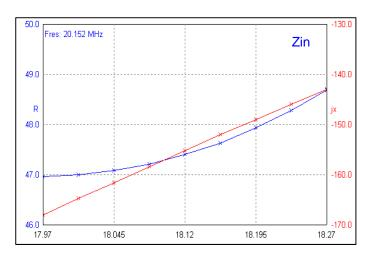
The SWR and Impedance graphs show that the G7FEK has an input impedance that is still relatively high on the 17 m band – with the SWR = 12.1:1, but it was easily tuned using an "T" match tuner. The antenna produces a number of lobes on this band and is no longer omni-directional. Moreover both the 40m & 80m antennas appear to contribute fairly equally to the radiation pattern.
