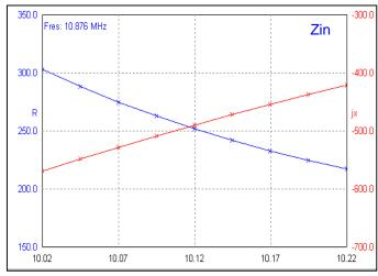
The MMANA MODELS SWR and Impedance graphs show that the G7FEK has a high input impedance on the 30m band – with the SWR = 24.2:1, but it was found that it could still be tuned using an "T" match tuner since the Autek VA1 measured the SWR = 2.5:1. The antenna appears to be omni-directional.
