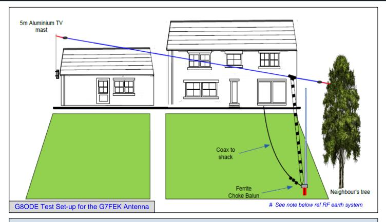
The test setup utilising a kind neighbour's tree as one of the supports. The other end is attached to an extended "TV" mast secured to the side of the garage. The G7FEK used the connection plate and RF earth of the disconnected 40m vertical antenna in the corner of the garden.
