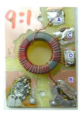
Next I tried a 9:1 impedance ratio UNUN. This an extremely popular impedance transformation ratio for end-fed or random wire SWL antennas. I wound 30 primary and 10 secondary turns on a FT114-43 ferrite torroid. The connection points are identical to those described in the above 4:1 UNUN. Remember that the impedance transformation ratio is the square of the actual turns ratio on your transformer; thus my 3:1 turns ratio is a 9:1 impedance ratio.
