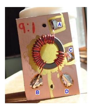
My experiments while constructing a reasonable quality MF and HF receiving antenna confirmed that using a UNUN, coax and a good RF ground system can reduce common mode RFI in my receivers.
