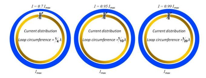
Clearly, the impedance (ratio of voltage and current) also varies around the loop; from highest at the capacitor, to lowest at the opposite point. So, for instance, there are two 50 ohm points, offset from the point opposite the capacitor (one on each side). This is used coupling methods such as Gamma Match and Delta Match.
