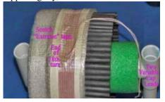
18) Refer to the photo at left. Using a sh scrap piece of waterproof tape, temporari tape the end of the 660/46 Litz wire leng the top surface of the Funnoodle material Leaving 10" of wire to be used for one or variable capacitor leads, start the first tur the Litz wire coil 2" from the right edge ferrite rods, as shown in the photo.
