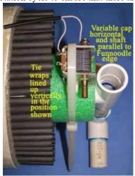
variable cap plates may temporarily brush up against the Funnoodle surface, but this will not affect the antenna's operation (shallow sections of the Funnoodle surface can be easily remove with sandpaper, if necessary). After ensuring that the variable cap is perfectly aligned and op smoothly, bend down the remaining variable cap upper terminal (next to the one soldered wir Litz wire) over the plastic tie wrap to lock the variable cap in place. Finally, cut off the exces wrap length.
