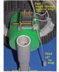
27) Refer to the photo below for the following step. Take the remaining 18" tie wrap and insert its end up through the right side tie wrap eye (as shown in the photo) for a length of 11", passing the tip in between the Litz wires and over the top of the variable cap, as shown.
