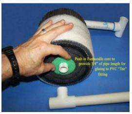
Note: PVC gluing operations should always be conducted outdoors (because of strong PVC glue fumes). It is also advisable to practice PVC gluing operations with scrap
