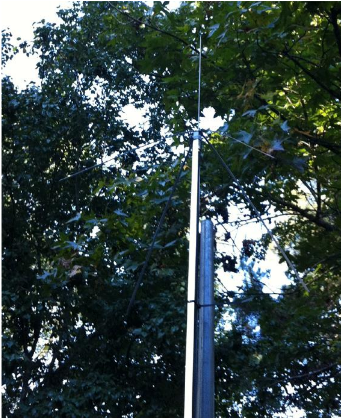
Mounted for testing. I spray painted the antenna a flat primer grey to protect it, and make it less reflective to blend into the background easier. These make great emergency antennas, stealth antennas, attic antennas, etc.
