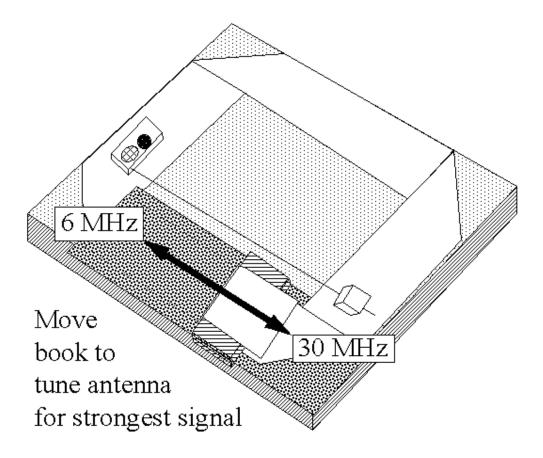
If you use a table model receiver (or an amateur transceiver,) make a single turn loop of about #18 insulated hookup wire by taping the wire in place one inch inside the foil loop. Bring the wire away from the antenna on the middle of the side opposite the tuner. Don't connect this loop to the foil - it isn't necessary.
