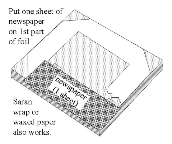
Leave the fifth flap of foil loose, so it can be lifted up when necessary. Cut off excess foil so it does not short circuit against the foil beneath the newspaper.
