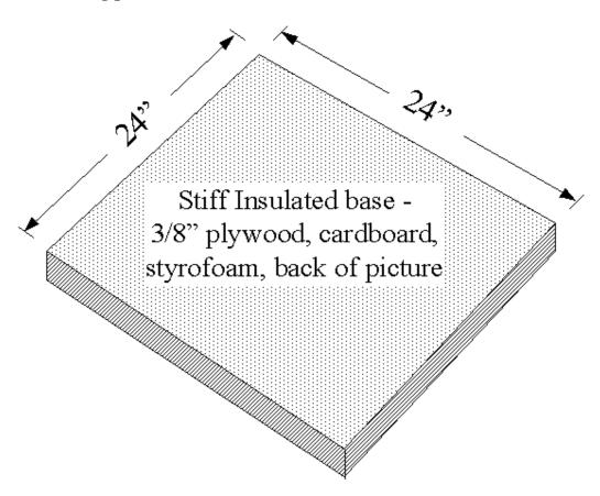
Cut a 6" wide piece of aluminum foil. Lay it on the base, with its edge along the edge of the base. Note the  $6\,1/2$ " gap where the foil begins.
