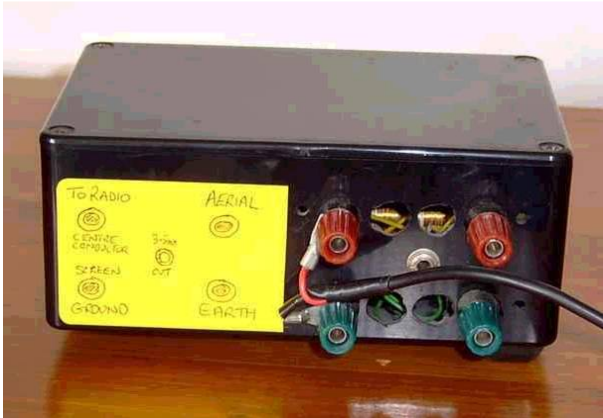
The rear panel of the Mk1 ATU showing the aerial input and output terminal posts. A 3.5mm jack socket is also included as an alternative output socket for convenient connection to a portable radio via a length of flexible 50 ohm coaxial cable
