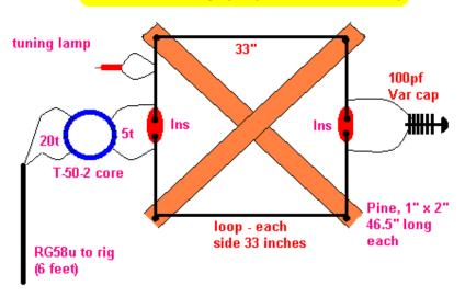
W9SCH described this small loop in Sprat 60 and it has proved useful to the QRPer, especially where space is at a premium.
