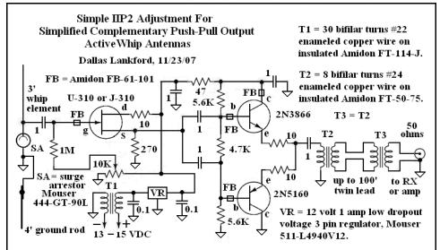
10 ohm drain resistor should be 1% all other resistors 5% or better, adjust 10K ohm pot for 0.200 volts across 10 ohm resistor using 2% accuracy or better DVM.
