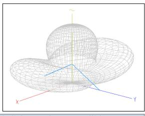
Antenna all modelled with the apex at 10m, over "real" ground = 5mS/m & dielectric =13 the apex angle set to approx 120 degrees.
