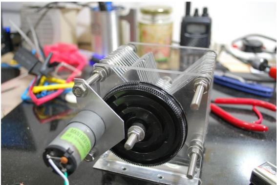
After some tinkering.... I decided to use a single cable for both RF and DC... I planned to make use of the FT897D ability to tune the antenna instead of having a separate box just to tune the variable capacitor. Since the FT897D has a built-in circuit to control the YAESU ATAS screwdriver antenna, it should be able to do the
