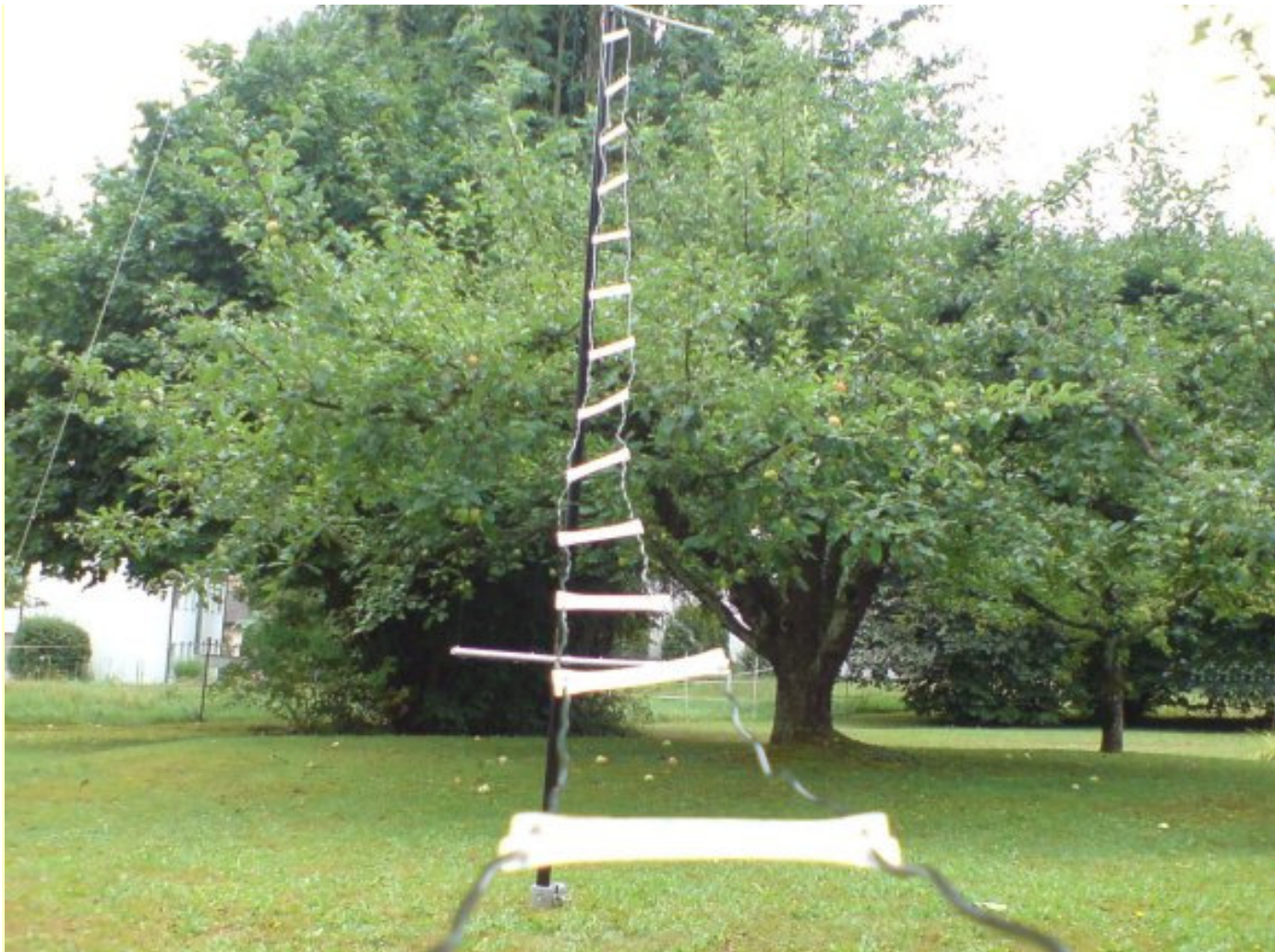
7.5 m homebrew ladder-line, 6 cm spacing, spreaders from Nylon sheet material
