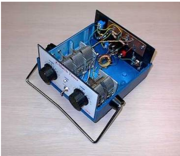
A different top view. Notice the N7VE SWR bridge is bolted to the back panel.
