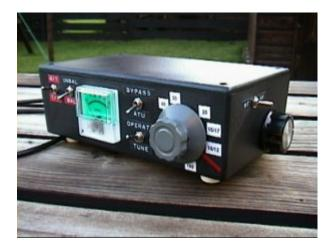
The ATU is built into a matt black box of ABS plastic having external measurements of 198 x 112 x 64 mm (Maplin part number BZ75S).
