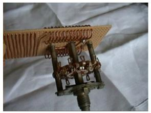
These pictures show the actual contruction of coils A; B; and C after having been mounted on the switch assembly, but prior to wiring.
