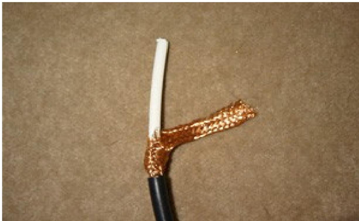
Pull the braid away from the center conductor and place some tape on the base of the braid where it separates.
