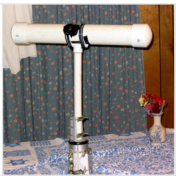
The antenna and rotor mounted on the clothesline pole in my back yard. I chose this location because it is away from power lines, houses, and the inverted L. However, the pole in the background carries some telephone wires, and I suspect that the null depth is compromised somewhat by re-radiation from these conductors.
