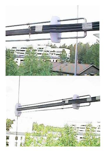
Connections are made 15cm (6") from the closed end of the stub. The stub is fed with a 50-200 ohm coaxial unbalanced to balanced balun. Using RG58 or URM76 the length of the loop forming the balun needs to be 0.33 x wavelength. A 1/2 wavelength radiating element for 145 MHz is 1030mm and the length of the coaxial balun should be about 690mm, folded to form a 345mm loop. You could, of course, simply roll it up!
