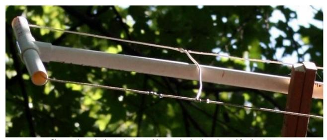
Shown above is the typical matching method using shorted feed points on the director #2 as an example. The reflector, and director #1 were done the same way. The driven element is fed with coax at it's respective matching point.
