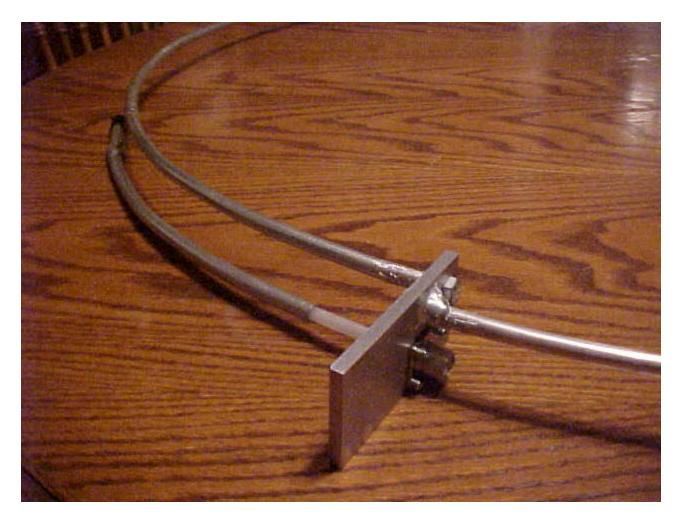
The so-239 connector is pop-riveted to the mounting plate. Face the pop-rivets out and away from the gamma section.
