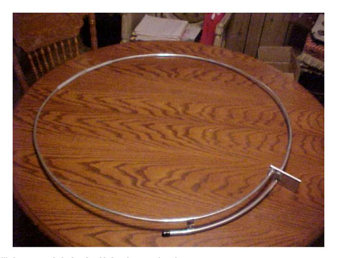
Both 54" elements are bolted and welded to the mounting plate.
