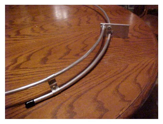
Position the 1" wide aluminum bracket on the Gamma arm, inward about 3 1/2".
