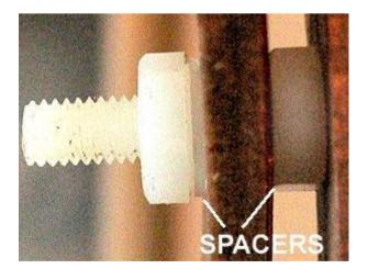
With the spacers located as shown, you can tighten the nuts so the loop tilts smoothly and easily, but doesn't droop when you let go.
