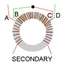
This drawing shows how the transformer is wound. I used different colors for clarity, but of course you can use the same color magnet wire for all windings; you'll only have to sort out the bifilar primary windings with an ohmmeter. Twist the bifilar primary wires lightly together. Two turns per inch is good enough. After winding, B and C are connected together and to the ground side of the secondary (connection not shown). A and D are the antenna terminals.
