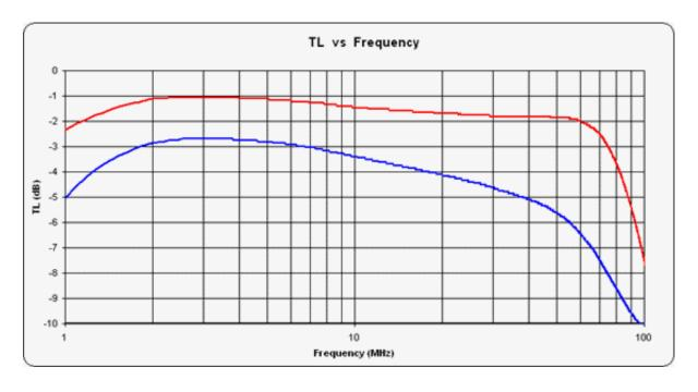
Graph showing loss through transformers. The Blue trace is the Comet clone and the Red trace is my improved
