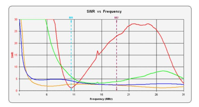
The graph above shows the VSWR measured at the base of a 6.5m high vertical supported by a 10m fishing pole. The Red trace shows the 6.5m wire fed directly. The Green trace shows a 300 ohm resistive termination, the Orange trace shows the vertical fed via a Comet style transformer, and the Blue trace shows the vertical fed via my modified version of the transformer. The two markers show the 1/4 resonant frequency (M1 at 10.5MHz) and the 1/2 wave resonant frequency (M2 at 21MHz).
