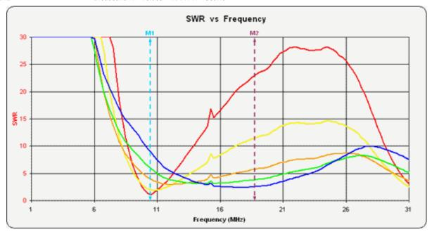
The Red trace is with a 50 ohm termination, Yellow with 100 ohm, Orange with 200 ohm, Green 300 ohm and Blue with 450 ohm. So the lowest overall VSWR is with a resistive termination impedance of around 200 to 300 ohms. The two markers show the 1/4 resonant frequency (M1 at 10.5MHz) and the 1/2 wave resonant frequency (M2 at 21MHz).
