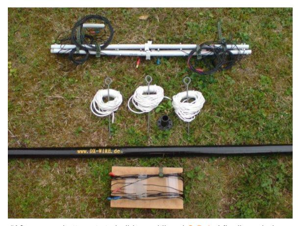
"After several attempts to build a multiband C-Pole I finally ended up with the Multiband H-Pole. C-Poles for different frequencies on one pole must be fed with separate feedlines over separate current baluns.
