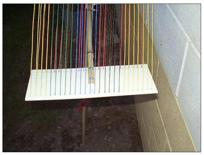
The loop wire is insulated, stranded stuff scavenged from long runs of security camera cables. THAT was a pain to strip and recover! I read that the ideal wire length for this kind of loop is 0.085 wavelength - which the total amount of wire turns out to be at 255KHz, pretty much band-centre of interest.
