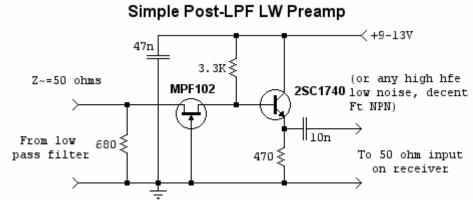
Circuit noise appears to be well below the noise level of the LW band, so that switching it in/out makes zero audible difference in the noise floor. No tuned circuits or coils... this is LF after all.
