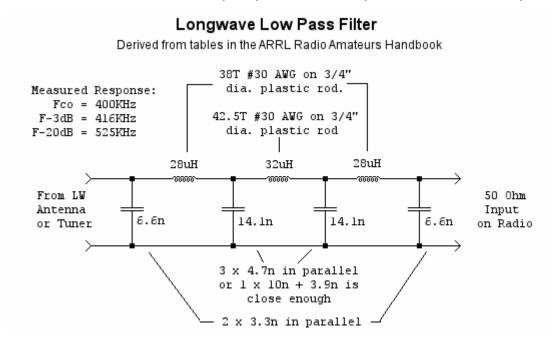
Coils are close-wound and easy to make from the plastic of a 3/4" knitting needle stolen from the wife and some RS wire. Note the orientation of the coils on the board (top of next page) so that they don't interact with each other. I hate using toroids for RF filters... you usually have to buy them, and that costs money.
