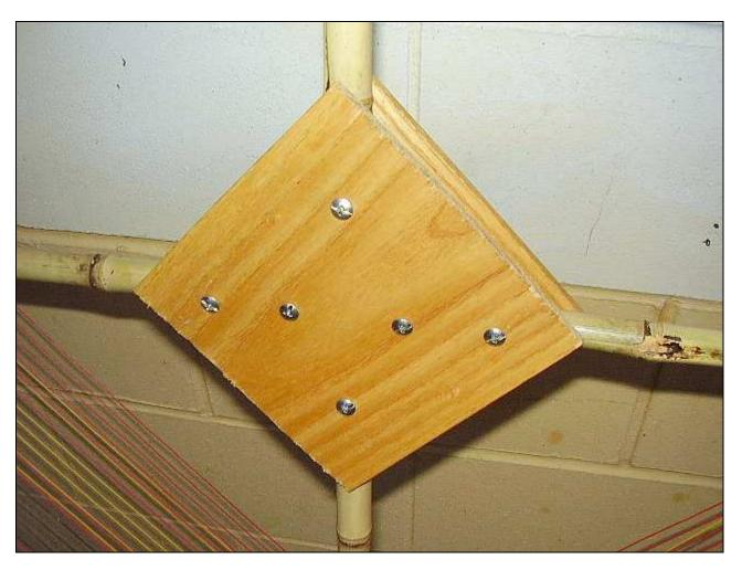
The hub plates are made from 3/16" ash thins for scroll sawing that I oiled for weather resistance. The arms and mast are formed from bamboo poles from a garden store. Strong and light!
