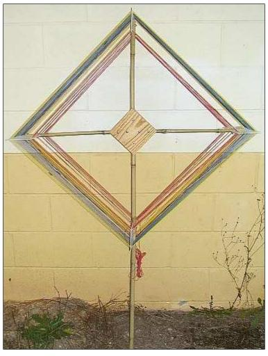
I just finished a small (69cm per side) quad loop for use from 150 - 430KHz that came amazingly close to the math prediction. I wound it for Non-Directional Beacon DXing...taking full advantage of the minimal sunspots recently, which makes for great LW DX.
