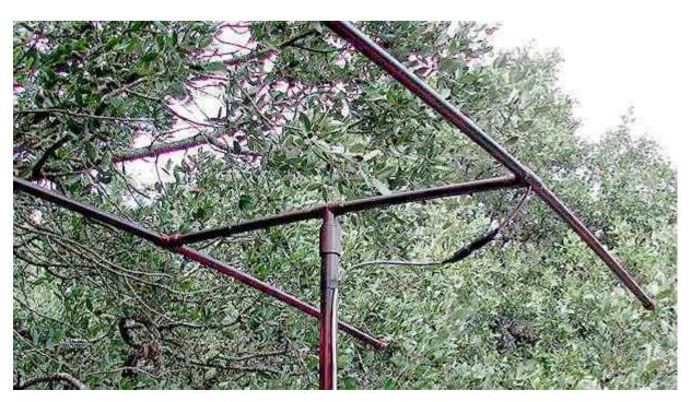
The 6 meter antenna has two elements and is housed in ½ inch pvc tubing, using T connectors to form the yagi configuration, and another T is located mid-way between the two elements for support. End caps are used to enclose the pvc ends. The coax feed is inserted into the DE T via a drilled hole on the T's under side. I used clear silicone to seal the hole.
