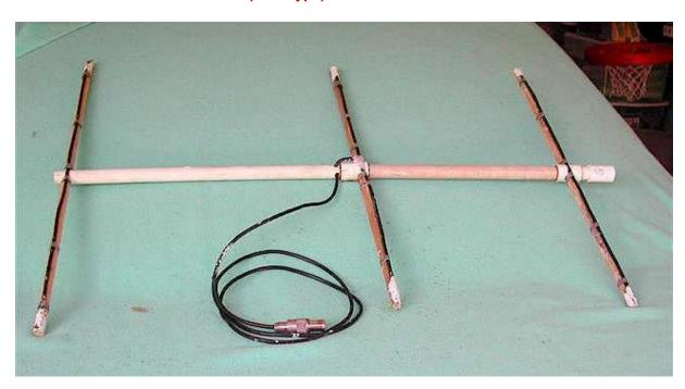
The 2 meter antenna in picture above is a three element yagi and again it uses John's formula for calculating the length for the DE and REF @146.0Mhz.
