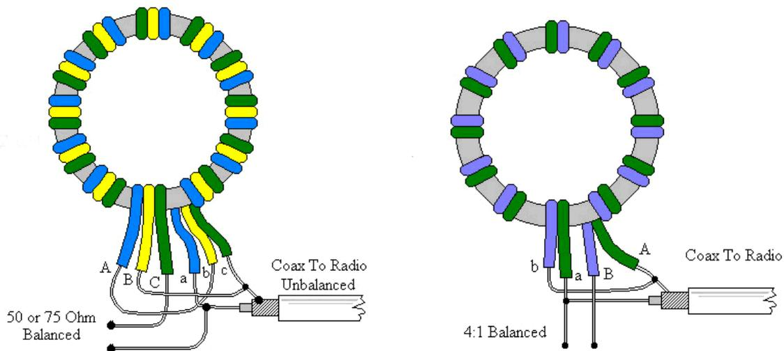
*Winding and connection detail.*
