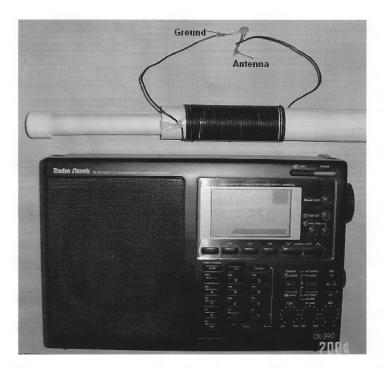
Notice that there are no connections to the radio. The AM booster sends the signals into the radio's internal par-core antenna. Position the top of the radio near the booster for maximum signal.
