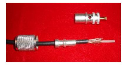
Slide the adapter down to the end of the black outer conductor. Then fold back the braid over the adapter.
