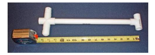
Glue the piece of PVC pipe into the Tee. Layout both pieces and mark the new pipe and glue it. From the hole in the top cap to the hole in the bottom cap should be 29"
