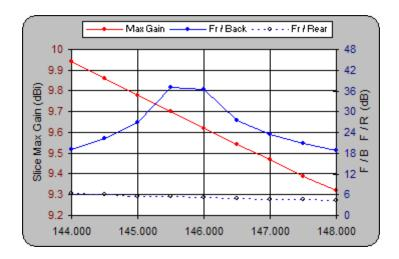
The chart shows the Max. Gain vs Freq. Notice at 144 Mhz. the Gain 9.95 and at 148 Mhz the gain is 9.3 dB.
