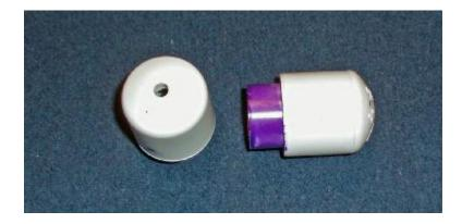
Drill a hole in the middle of the Cap with a size # 17 drill.
