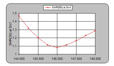
This is the calculated SWR curves for our antenna. Notice it covers the entire 2M band with an SWR of less than 2.
