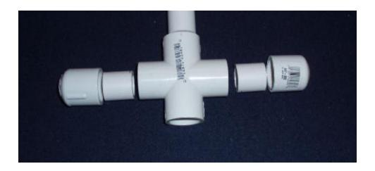
Coat the pieces with the PVC cleaner (purple solvent). Coat the inside of the Cap with the PVC glue and insert the short piece into the Cap approximately half way.
