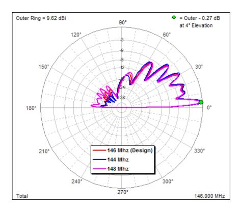
Plot of Signals perpendicular to the ground. This is also where we get the radiation angle.
