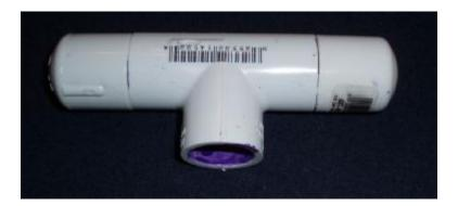
Mark the ends for the center spacing. These marking will be used later to mark the wire so we know how far inside the fitting the wire extends. This is a pretty precise measurement if you want to get the best out of the design.
