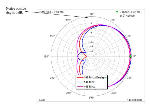
Antenna Pattern parallel to the ground – notice the large beam width.
