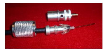
Screw the adapter into the PL-259. Now we are ready to solder. You will need a large high wattage soldering iron for this. The small pencil types are not large enough and the PL-259 acts as a heat sink. By the time you get the solder to flow you might have melted the center conductor. I use an old Weller 550 watt soldering gun.
