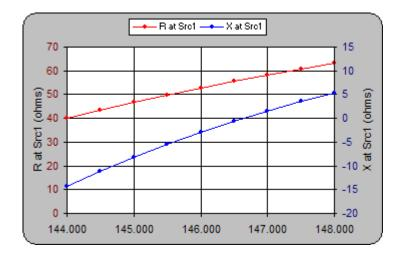
If the antenna was a 50 ohm resistive circuit then the SWR would be 1:1 but because we have SWR the Impedance and the Resistance changes across the band. Notice at the design (146 Mhz) the resistance is close to 50 ohm. Most antennas never are perfect 50 ohm resistive. As they move off resonance then you start to get some Impedance.
