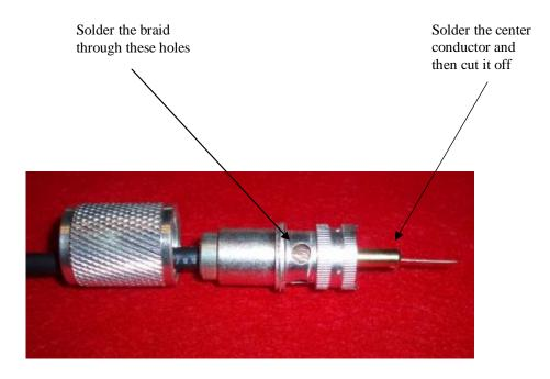
Notice how the solder is flowing. *If the solder doesn't flow you don't have a good soldering connection.* You only have to solder a couple of the holes and the braid.
