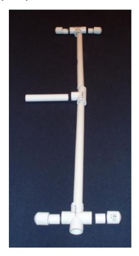
Making the end assemblies. They consist of 2 -  $\frac{1}{2}$ " PVC Caps and 2 – PVC pipe sections ~  $\frac{3}{4}$ " long.
