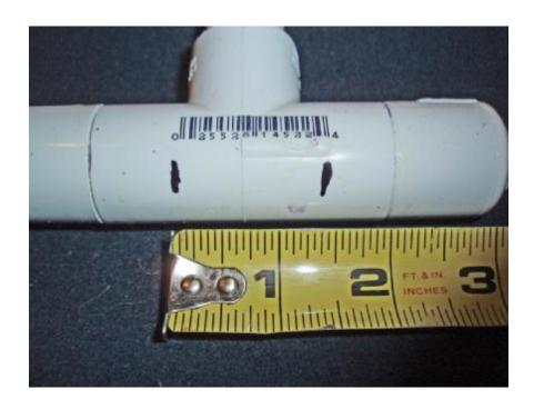
When both end have been marked assembly one half of the antenna. Measure the length between the middle and the center of the cap. This will provide a good performing antenna. The antenna is 29" long so you should have 14 ½" from the center to the hole in the end cap. I turned the Tee so I could get a good measurement and marked the pipe. I turned the Tee around correctly and glued the Tee onto the pipe.
