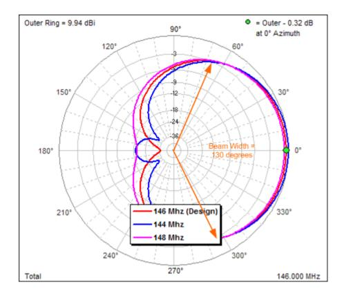
Another measurement for beam antennas is the Beam Width. This is defined as the width of the radiation beam where the power is reduced by 3 dB (half power or half power points). The Moxon has a very good beam width in that if you are anywhere in the front of the antenna you have a good - fair signal, once you go to the back side the signal is very reduced. You can use this characteristic to remove strong signals from different locations.
