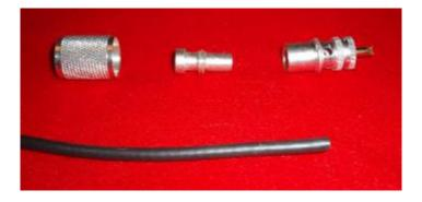
We will use a PL-259 and an adapter. If you are using RG-8 then no adapter is needed. There are several different adapters that you can use. You have to purchase the correct adapter for the cable. RG-58 uses a different adapter than RG-8X (mini – RG-8) or RG-59.
