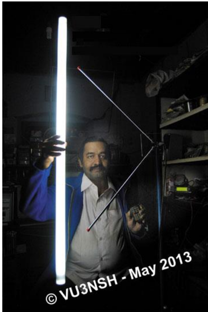
Fig. 6. RF radiation test by VU3NSH with tilted V antenna
