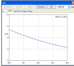
The SWR plots show that the FD3 antenna has a low SWR on 20 & 10m band, and that for these bands there is an upward shift of the resonant frequency due to end effects. The 40m SWR results indicate that some antenna matching is required due to ground reflections because the antenna is lower than a quarter wavelength on this band. The far field plots also show that this low height affects the overall shape and the number of lobes that are created and hence, the take off angle.
