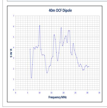
The SWR plot on the left is for my homemade FD3 using a Moonraker<sup>Tm</sup> 4:1 400 watt current balun. Three clamp-on ferrites were added at the top of the 12m long Mini-8 coax feeder I use to connect my remote antenna relay box. The SWR measurements were taken at the end of the Mini-8 coax using an Autek<sup>Tm</sup> VA1 antenna analyser.
