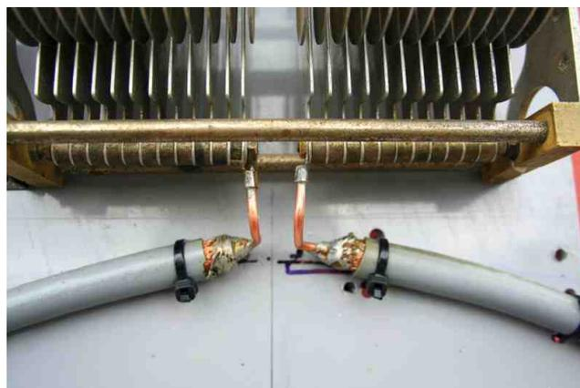
Connection of loop ends to capacitor.
