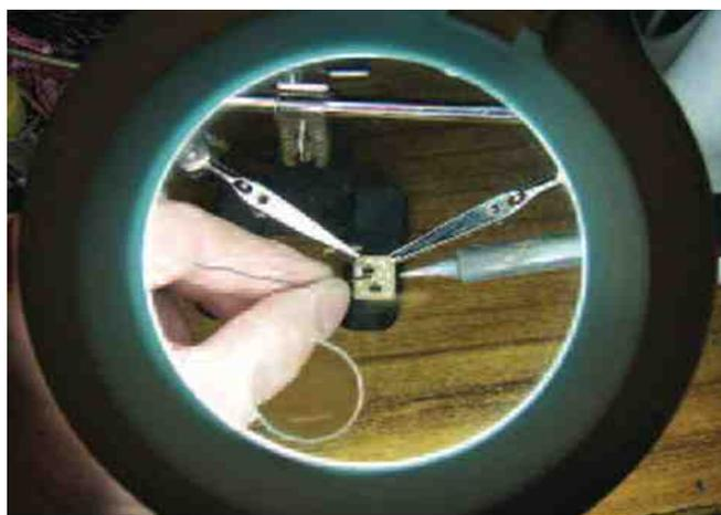
PHOTO 5: Soldering surface mount devices is often more easily accomplished with the aid of a strong magnifying glass
