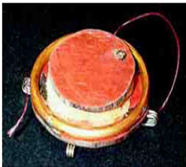
Figure 5—The assembled microphone element.
