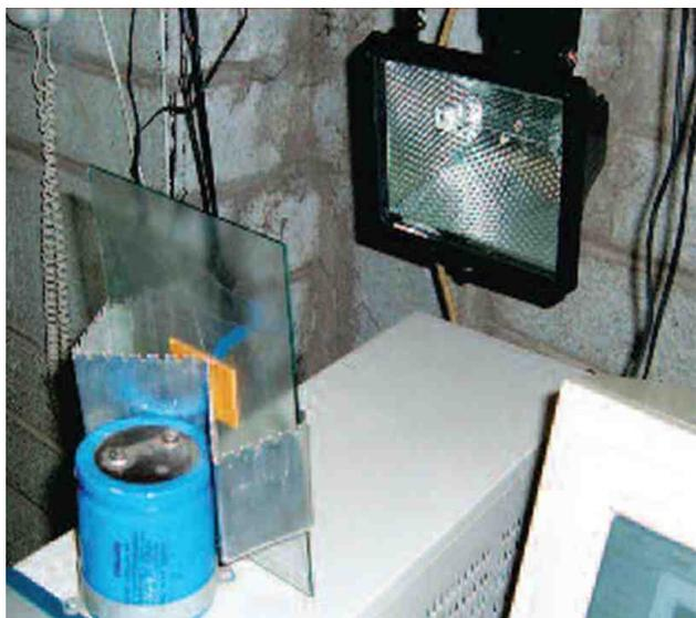
PHOTO 2: My not-so-high-tech PCB exposure system
