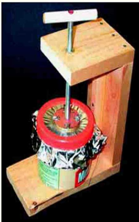
**Figure 6**—Applying the aluminum foil diaphragm to the element using a homebrew test fixture. Notice the bead of epoxy cement around the edge of the spacer ring. The diaphragm is held in this position until the glue dries fast. It is then trimmed, close to the ring.
