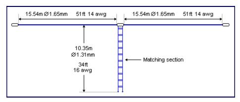
The antenna may also be used in the form of an inverted-V ( $\Lambda$ ). However, it should be borne in mind that, for such a configuration to radiate at maximum efficiency, the included angle at the apex of the  $\Lambda$  should not be less than about 120° (although many authors consider an opening between
