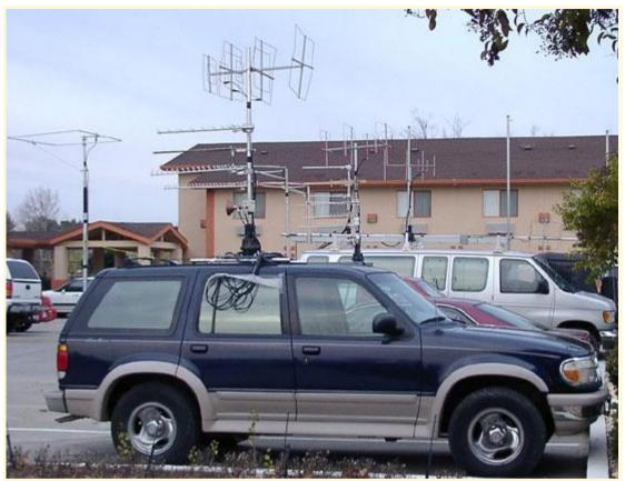
This photo shows the antennas on three rover vehicles the morning after the January, 2004 VHF SS contest. All of the antennas took hits during the contest, tangling with at least one tree each. The 3-element 144, 222 and 432 MHz triband quads are atop rotating masts, with antennas for higher frequencies below them.
