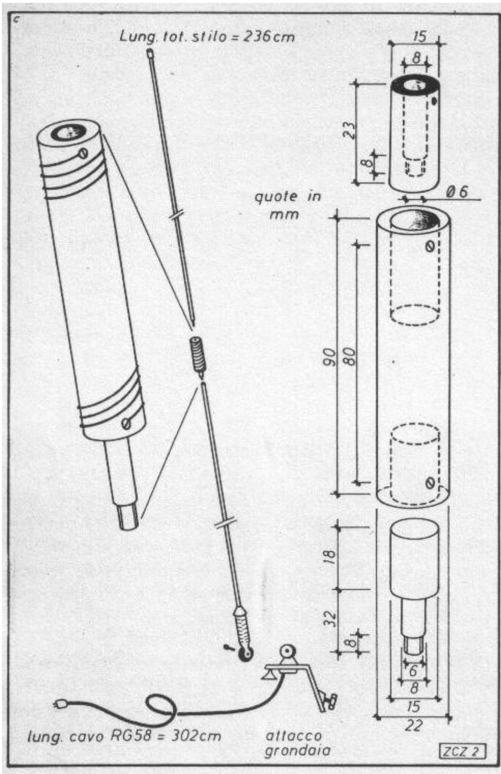
10m = no coil ; 15m = 22 turns (spaced), 1mm wire diam, coil length = 80mm ; 20m = 37 turns same wire and coil length.
